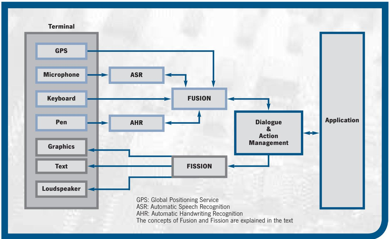
Figure 5: Schematic diagram of the modular architecture of a multimodal service.
